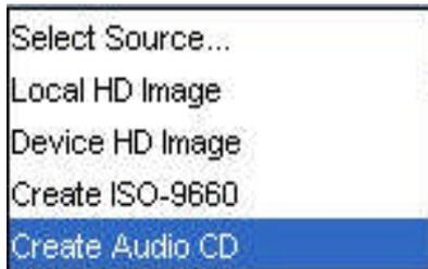
'Create Audio CD' will enable the user to build an Audio CD from suitable WAV files located on the local HD. No image is created on the local hard disk. If you want to keep the Audio CD image for later use, select the Audio CD button on the toolbar instead, then select this built image when starting a job. See Audio CD creation for more details.
