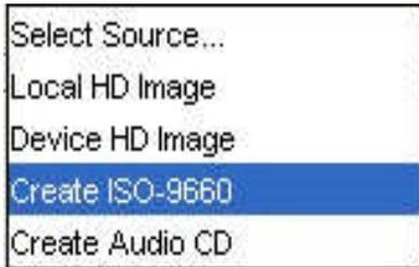
Selecting 'Create ISO-9660' will launch the ISO create dialog that allows you to specify a source directory path. When selecting this option, a 'virtual' image is created and sent to the Network Device. No image is created on the local hard disk. If you want to create an image file to keep for later use, select the ISO button on the toolbar instead, then select the built image when starting a job. See creating ISO images for more information.
